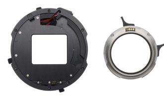
Rear view of LPL Mount (the side that attaches to the Sony VENICE body with six screws. Lens data contacts are at the 6 o'clock position.) Above right: rear of LPL to PL Adapter, showing PL lens data passthrough.
